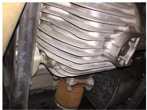
Torque 33 lb/ftDrain bolt. 24mm. Torque 33 lb/ft
